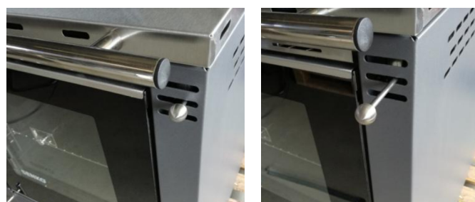
Closed flue gas deflector (17) Open flue gas deflector (17) ⇒ Boiler efficiency significantly reduced!
