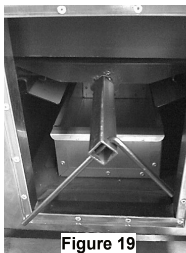
firing regime adjusting mechanism with regime adjustment spanner (24)
