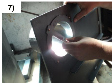
7) Afterwards, connect the chimney extension to the protective round cover and re-tighten the previous four bolts
